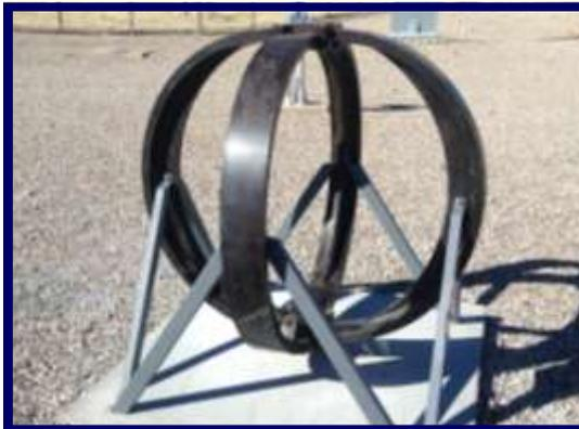
*The SLFCS antenna is actually two antennas. The hoops are about six feet across.*
